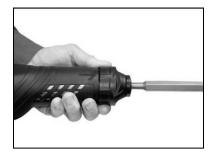
The chisel can be fixed in 12 positions. Pull the fastening ring of the chisel forward and turn it. In the desired operating position release the fastening ring to its initial position.
