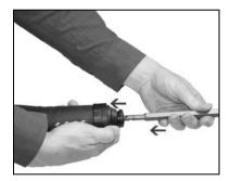
For removing the chisel pull the locking sleeve backwards.
