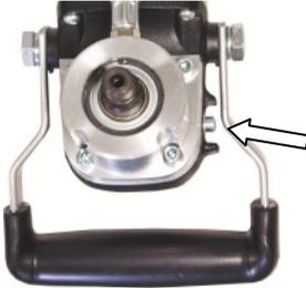
Actuate the spindle stop and keep it pressed. Mount or remove the tool.
