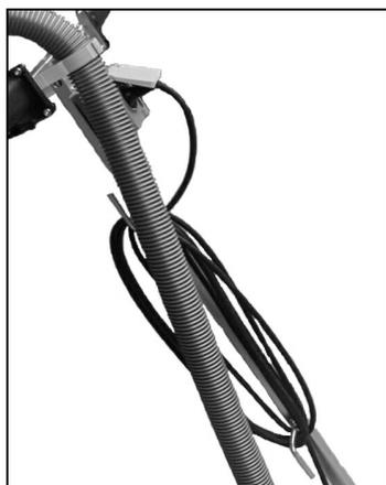
Wind the line cord of the tool on the holder meant for this purpose. **Make sure that the switch of the floor guiding device is not pressed or locked.** Plug the grinder in the socket of the floor guiding device. Lead the hose of the vacuum cleaner above the floor guiding device, connect it with the grinder. The clamp will avoid a slipping of the hose.
