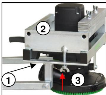
Then put the device with the holder (1) under the frame handle and fix it with disc, spring ring and wing nut (3) on the top frame (2).
