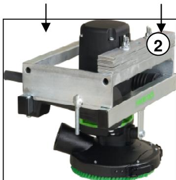
Put the top frame with the weights (2) on the frame handle of the machine.
