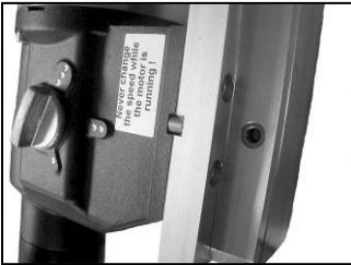
The tool is supplied with a mounting plate, a 10 mm fitting key and 4 Allen screws M8x30. The mounting plate is put on the drill motor with the fitting key and fixed by means of the 4 screws.
