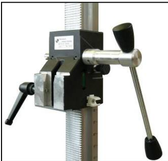
The machine holder has a special quick connection fixture for the machine ETN 152/3 P. Thereby the prism on the gear box of the machine will be insert from above in the dovetail fixture of the machine holder and braced firmly with a laterally clamp lever.
