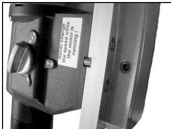
The tool is supplied with a mounting plate, a 10 mm fitting key and 4 Allen screws M8x20. The mounting plate is put on in such a way with the fitting key on the machine that the socket is in the mounting plate on the same side as the gear switch of the machine. Afterwards the four screws are insert and tightened firmly.
