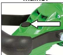
Actuate the spindle stop and keep it pressed.
