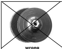
Press the grinding wheel which is necessary for your application on the sanding disc with velcro-type fastening. Pay attention that the sanding disc is well-positioned on the tool, in fact as exact as possible. This allows a quiet run of the machine.
