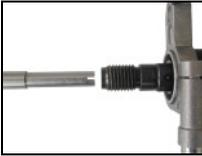
Insert the centering rod so that the recesses in the centering point latch on the catches of the working spindle.
