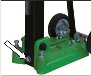
Remove the screw, which locks the column at 90°.
