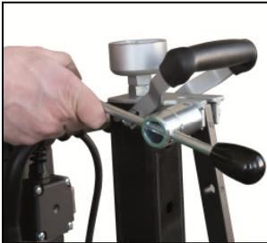
Open the top screw of the support with the turnstile.
