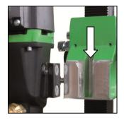
Block the tool slide by means of the knurled screw. Insert the tool into the drill rig. Fix the tool by close the screw.
