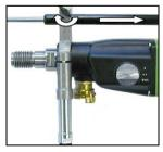
Insert the gas spring with the water collecting ring and the guide ring appropriate for the drill bit diameter into the tension disk. Shift the gas spring up to complete coverage of the bit segments by the water collecting ring. Tighten the wing screw. On drilling overhead, make sure that the water supply is opened only after having switch the water remover on and the removing unit was fixed to the wall or ceiling.
