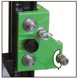
Open the fixing by turning the screw in direction of the arrow until the guideway is free.
